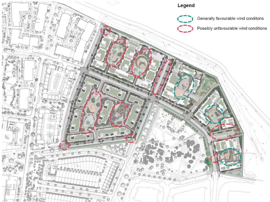
Diagram showing wind conditions expected following specialist wind analysis, prior to mitigation by landscape.
